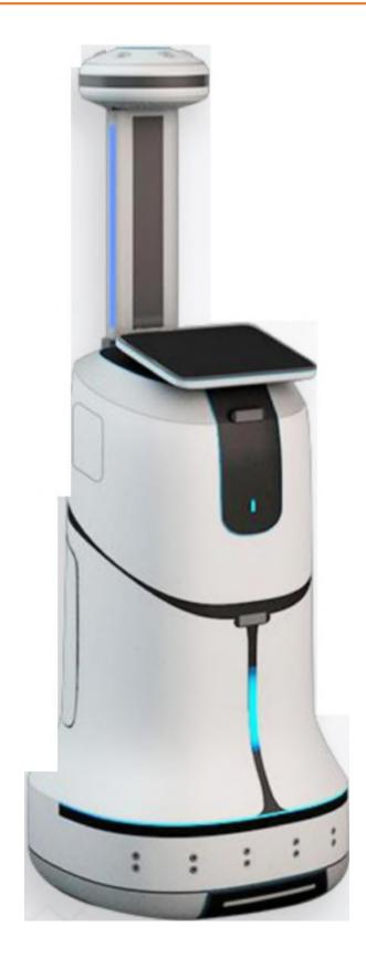
Intelligent dry fog robot can atomize a variety of disinfectants, and through the high-speed air will fog After the fog drops dispersed to the disinfection area, the realization of disinfection. The robot can navigate and avoid obstacles autonomously And the way to move to the disinfection area, around the disinfection target for 360 degrees without dead Angle disinfection. At the same time, I Pad remote control is supported to rapidly and centrally sterilize the area.
