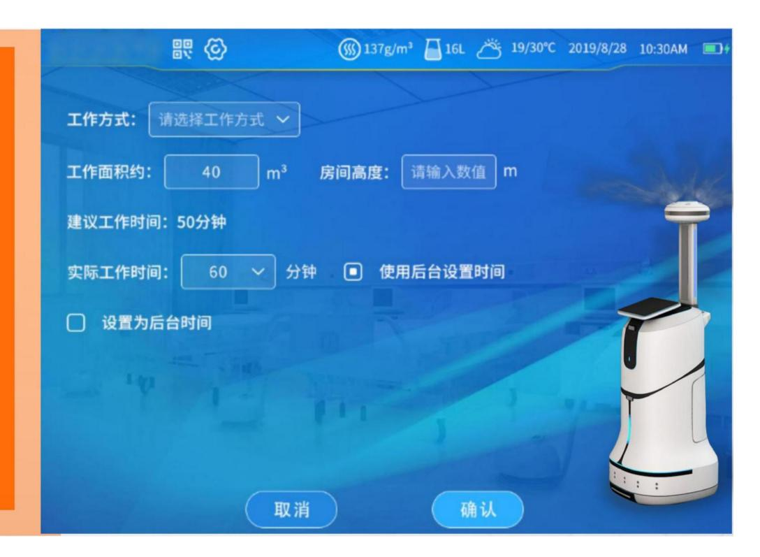
The robot can calculate the best operation time according to the regional space situation. If the operation area changes, it can adjiust the regional space parameters at any time to ensure the best disinfection effect. Moreover, it can save the job record to the cloud server, which is convenient for direct use next time, fast and efficient.
